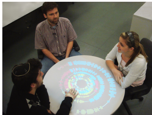
Figure 1. The Conversation Clock captures conversation via microphones to demonstrate patterns of interaction. Past studies have shown that collocated conversation tends to balance in response to the visualization's presence. In this work, we appropriate the visualization for remote use to examine the effects of a distorted visualization on conversation.
