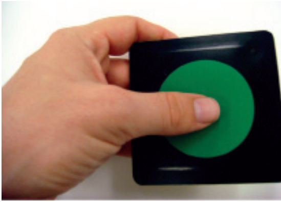
Figure 7. The green button from the first iteration of the conversation votes table. Pushing this button indicated agreement with the current speaker; pushing the red button indicated disagreement.
